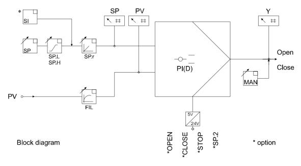
**Setpoint limiting**. Minimum value SP.L (setpoint low), maximum value SP.H (setpoint high). Only setpoints within the setpoint limiting can be set via front keyboard.
