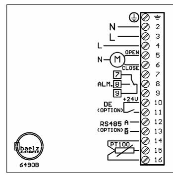
Wiring diagram 6490B, 6490B-y and 6590B
