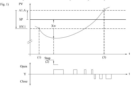
After the plant has been switched off, the temperature in the tenter has to drop below the hysteresis of the alarm relay until the control of the burner is released again (1).
