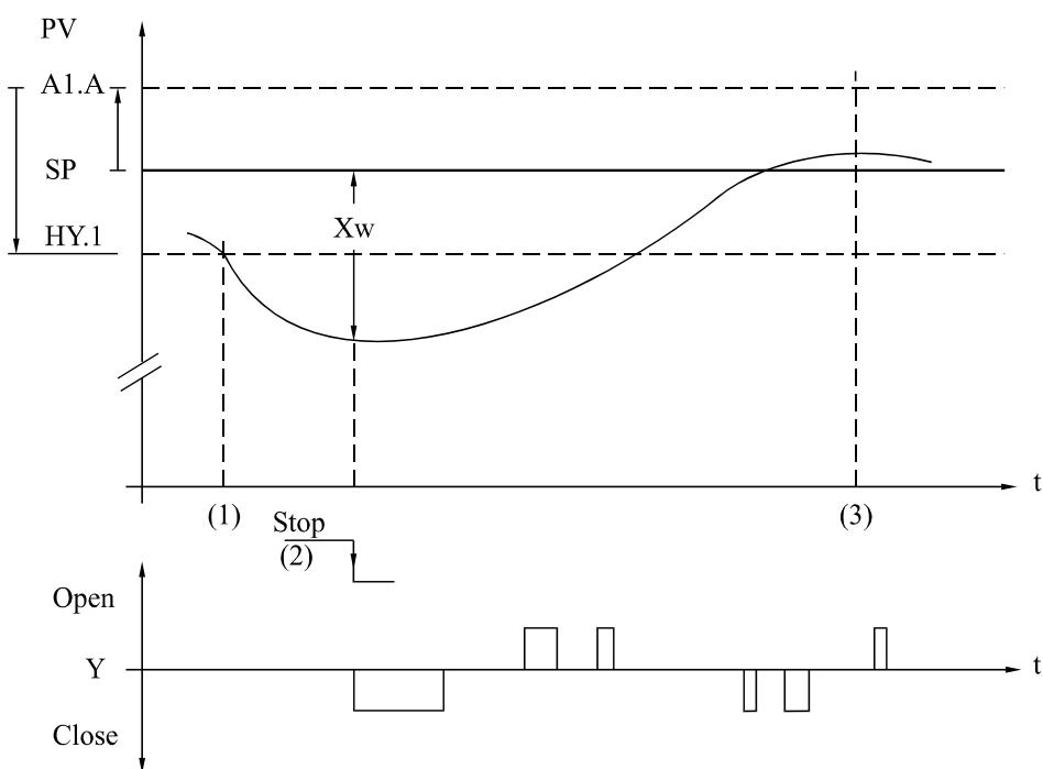
Because of the delta setpoint, as soon as the STOP command is inactive, the first OPEN pulse is either shortened according to the adjusted setpoint lowering and the control deviation  $X_w$ , or a CLOSE pulse may even be given (2).
