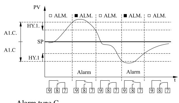
**At all three types (A, B, C) alarm is always triggered in case of sensor failure.**
