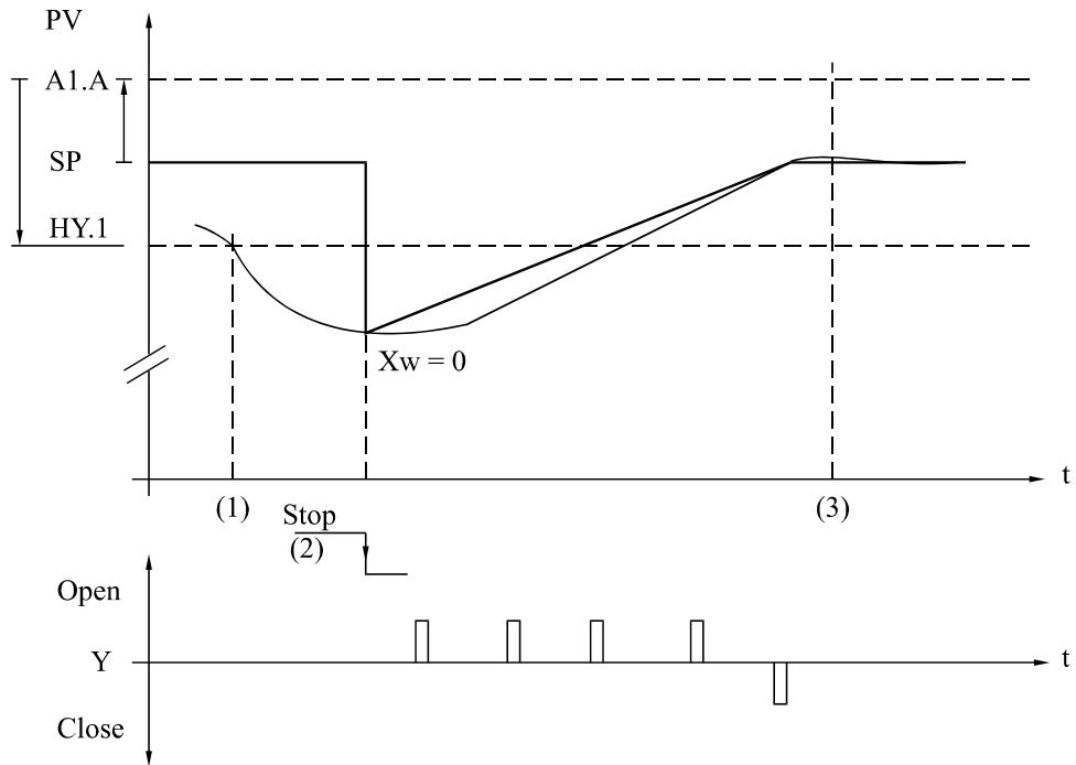
A soon as the STOP command is inactive the setpoint SP is automatically equated with the current temperature PV (2).
