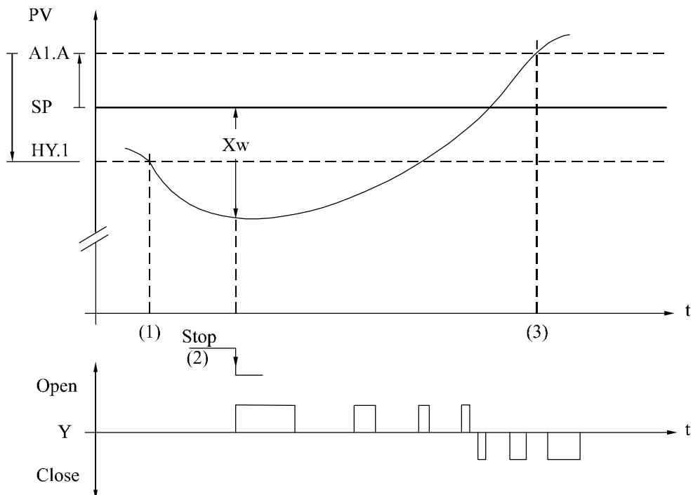
After the plant has been switched off, the temperature in the tenter has to drop below the hysteresis of the alarm relay until the control of the burner is released again (1).
