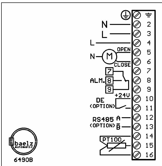
Wiring diagram 6490B, 6490B-y and 6590B
