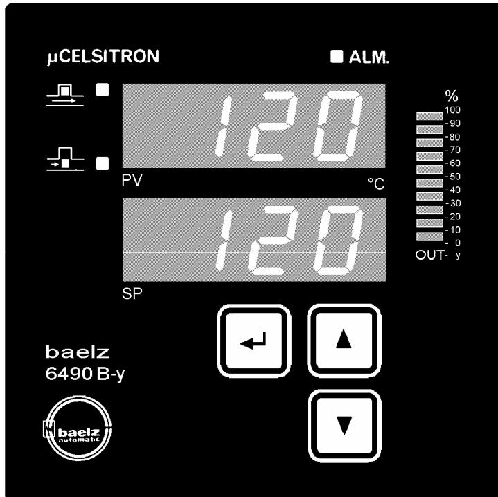
The bargraph displays the manipulated variable Y in 10% steps:
