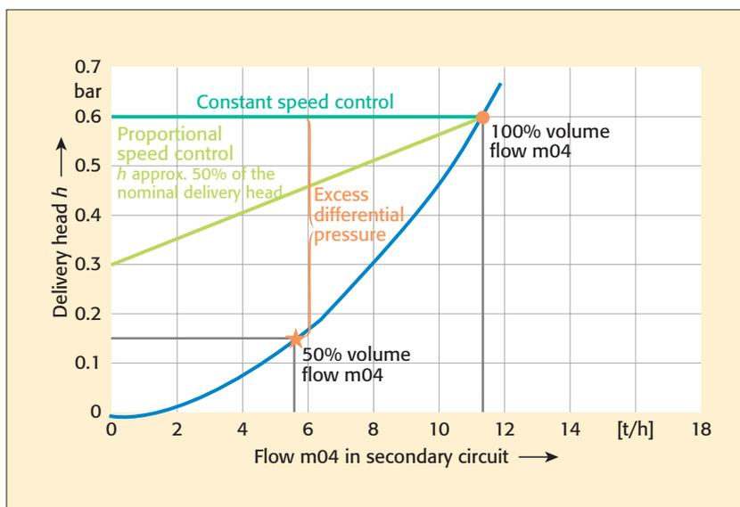
Figure 4. Pipe network characteristic (blue) and pump characteristics (green)
