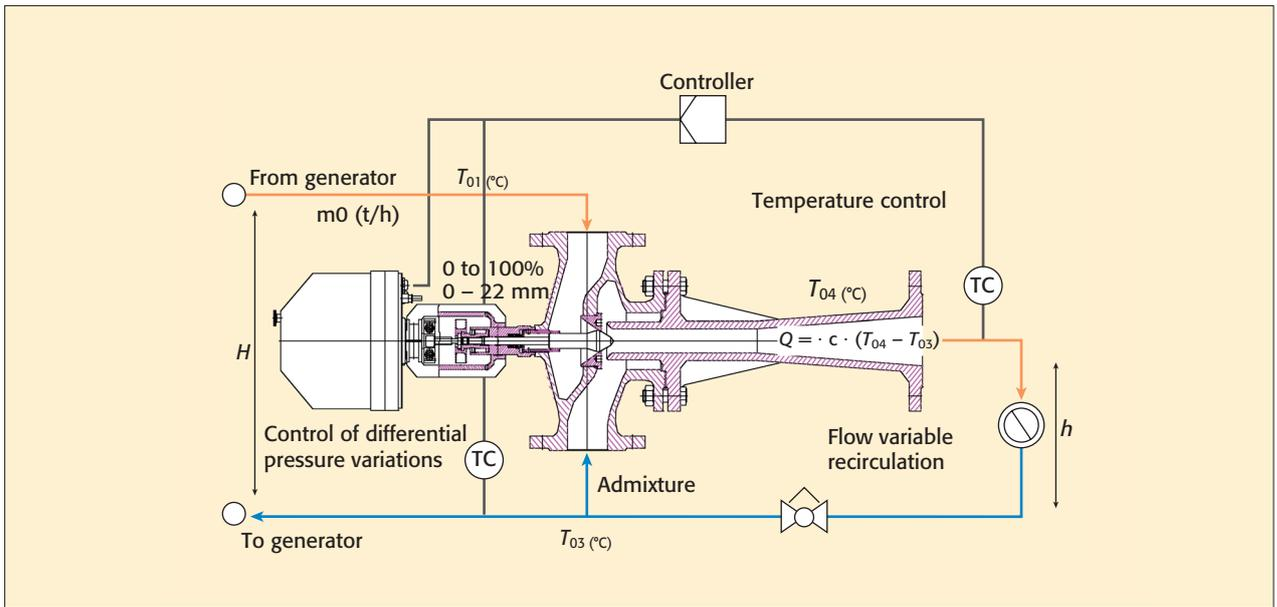
Figure 8. Functional diagram of the ejector system
