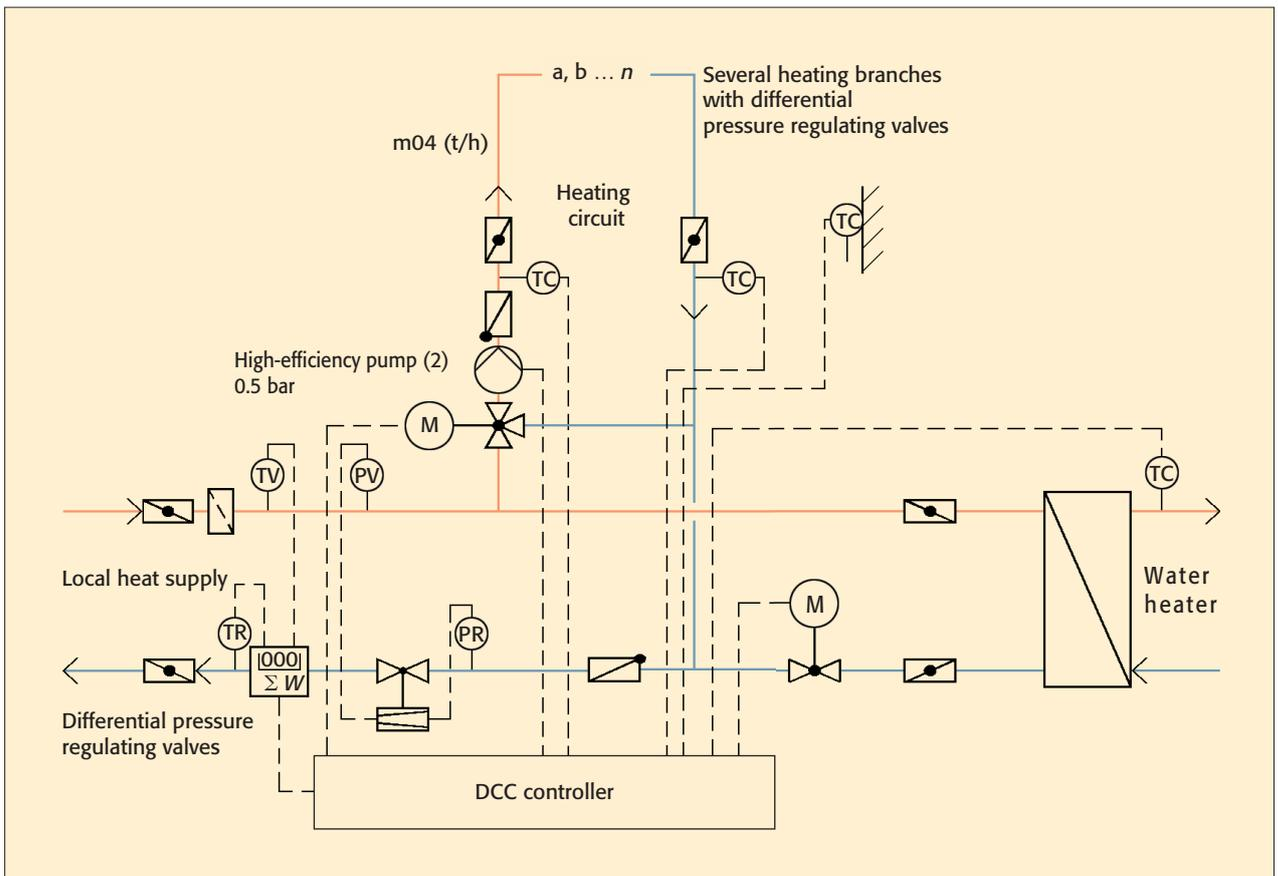
Figure 3. Building heating system installation with inefficient design
