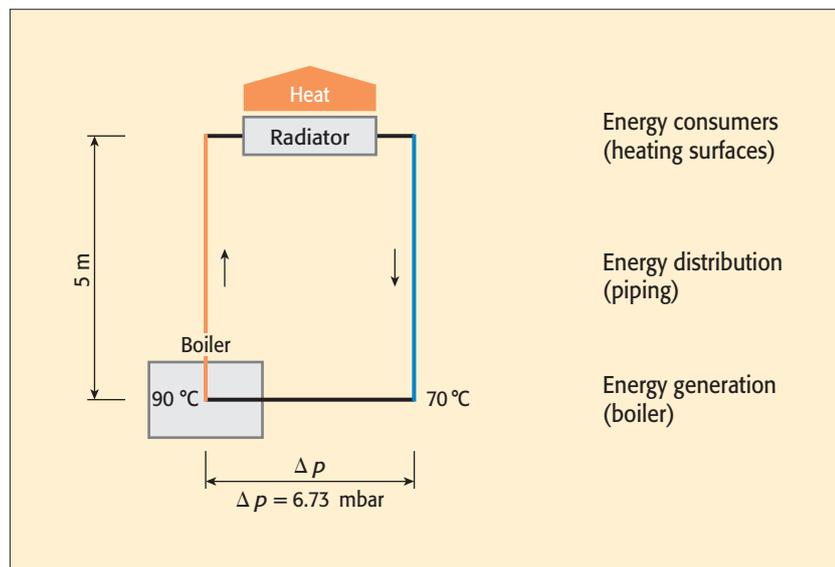
Figure 1. Gravity heating system
