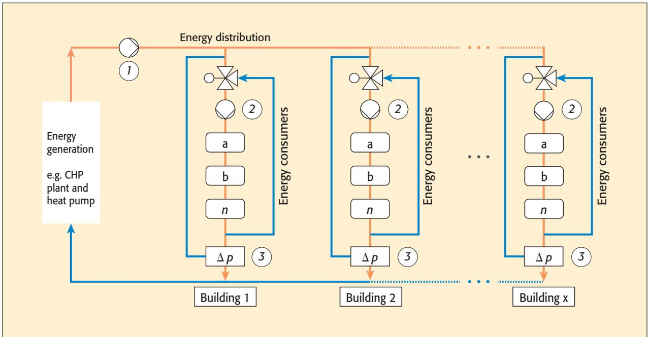
Figure 2. Complete system with inefficient design
