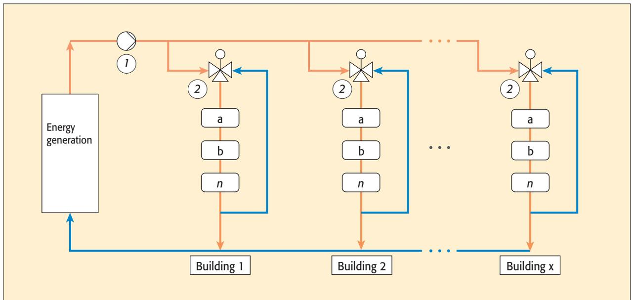
Figure 5. Control with ejectors
