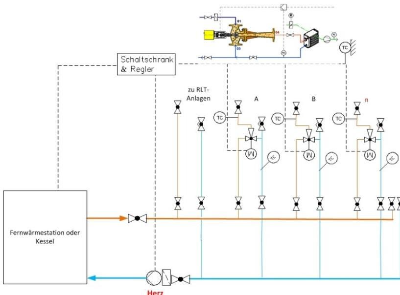
**Figure 1** System design for heat and cooling distribution at Vivantes Berlin Hellersdorf 2015
