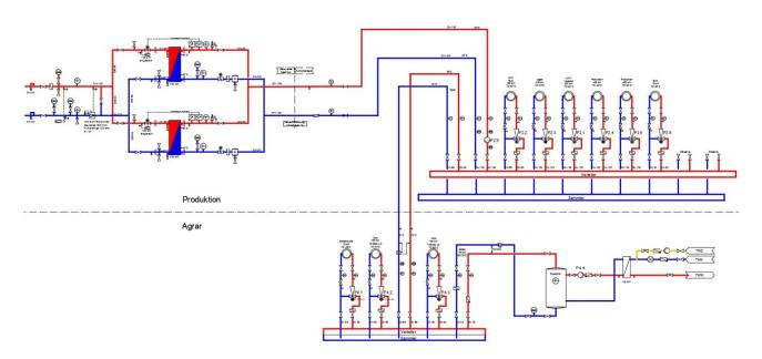
Figure 3 New system layout after modernization for Agriculture and Production
