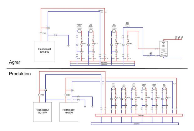
Figure 2 Old system layout before modernization for Agriculture and Production
