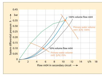
Figure 7. Pipe network characteristic curve when using a controllable ejector
