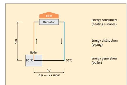
Figure 1. Gravity heating system
