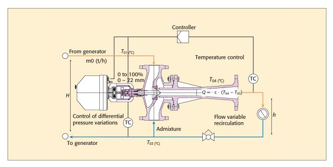
Figure 8. Functional diagram of the ejector system
