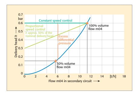
Figure 4. Pipe network characteristic (blue) and pump characteristics (green)
