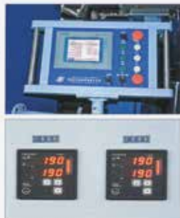
温度产线控制 Temperature control panel for stenter
