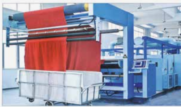
卷布系统 30寸开式卷布及送布机 Delivery system 30 inch with a feeder for width roll
